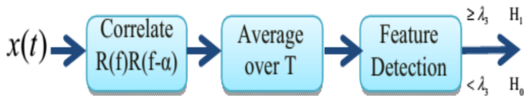
Figure 1. Block diagram of cyclostationary detection
